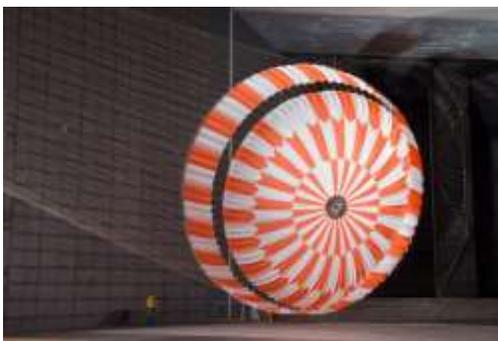
**Testing Perseverance’s Parachute:** The enormous supersonic parachute for the Mars 2020 mission undergoes testing at the world’s largest wind tunnel at NASA’s Ames Research Center. Credit: NASA/JPL-Caltech/Ames. [Full image and caption >](#)
