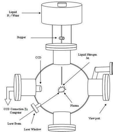
Figure 1: Schematic of Experimental Setup
