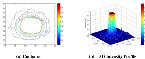
Figure 5: Contours of Liquid Nitrogen plasma along with 3 D Intensity Profile.
