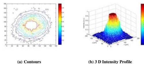
Figure 6: Contours of Water plasma along with 3 D Intensity Profile.
