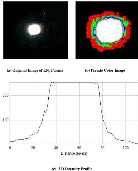
Figure 2: Images of Liquid Nitrogen Plasma along with Intensity Profile.
